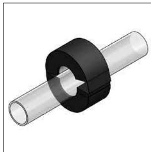
Position insulation body on pipe
