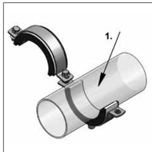
Position pipe in insulated pipe clamp
